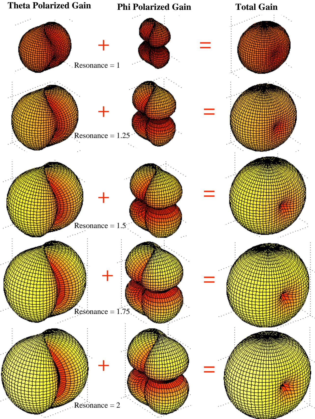
Figure 8 Far field radiation patterns for typical CTHA at various points of a normalized spectrum.
