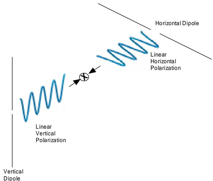
Figure 11 Orthogonal dipoles do not communicate.
