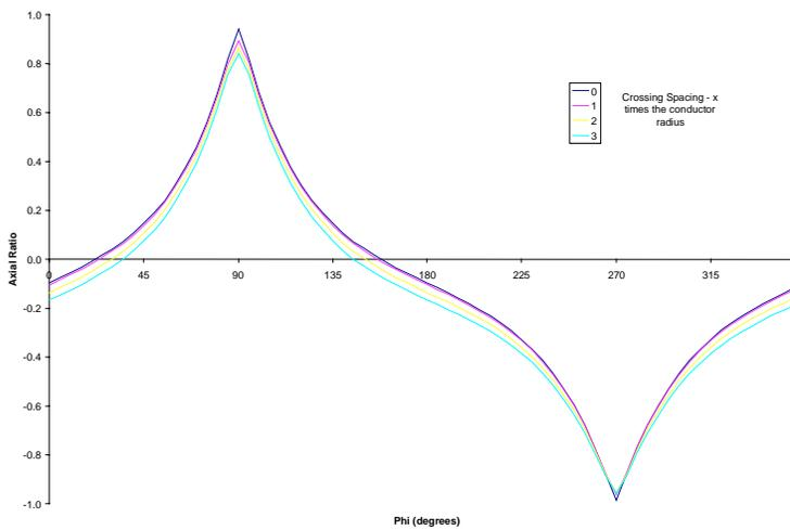
Figure 13 Axial ratio at theta of 45 degrees for several CTHAs with different cross-over spacings.
