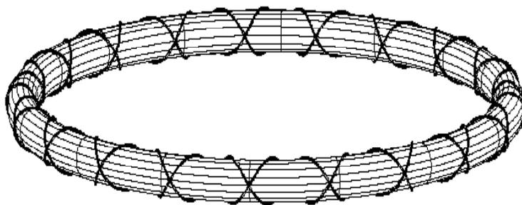
*Figure 1 A Contrawound Toroidal Helical Antenna.*
