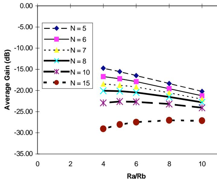
Figure 14 The effect of number of turns and  $R_a/R_b$  on relative average gains.
