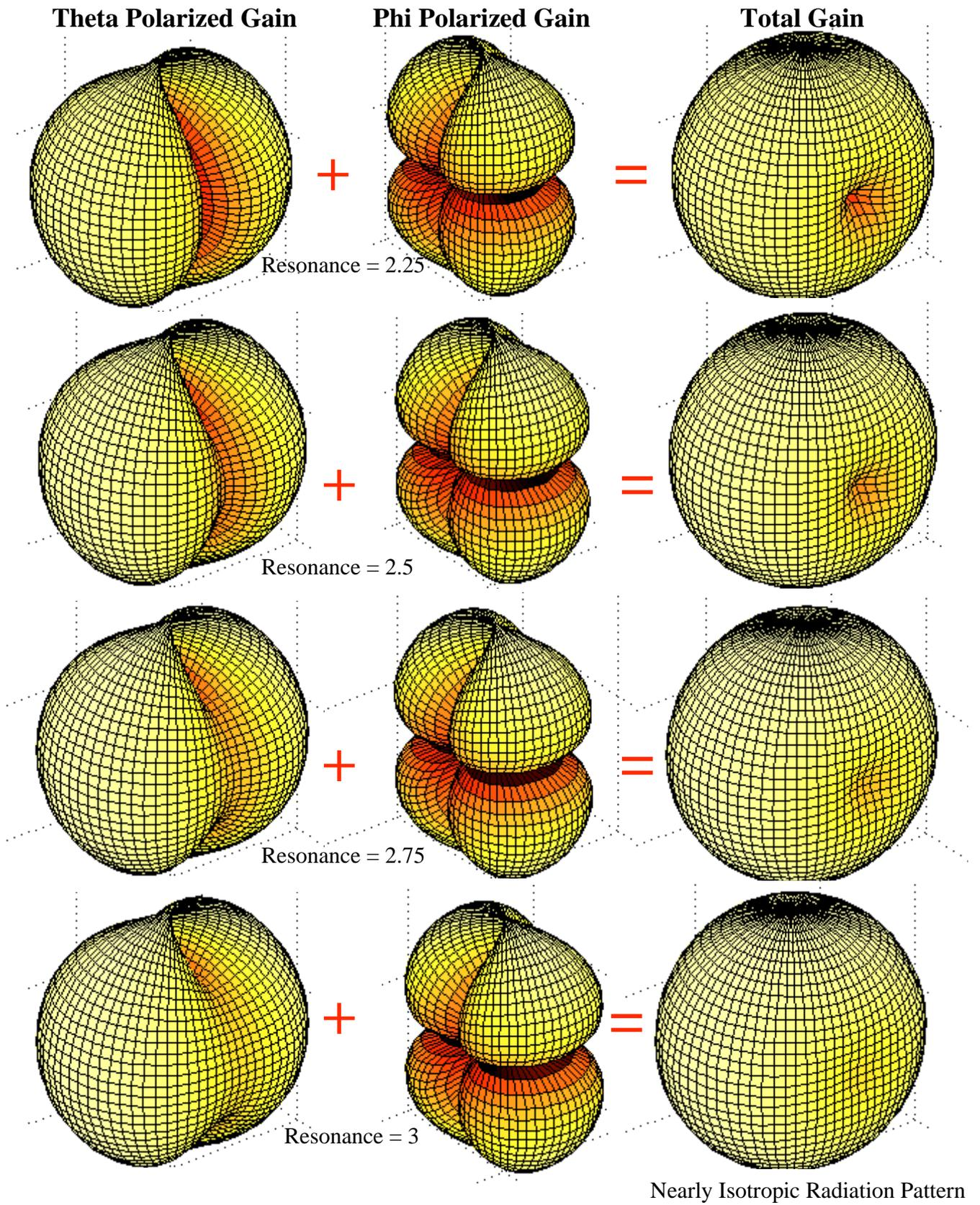
Figure 9 Far field radiation patterns for typical CTHA at various point of a normalized spectrum.
