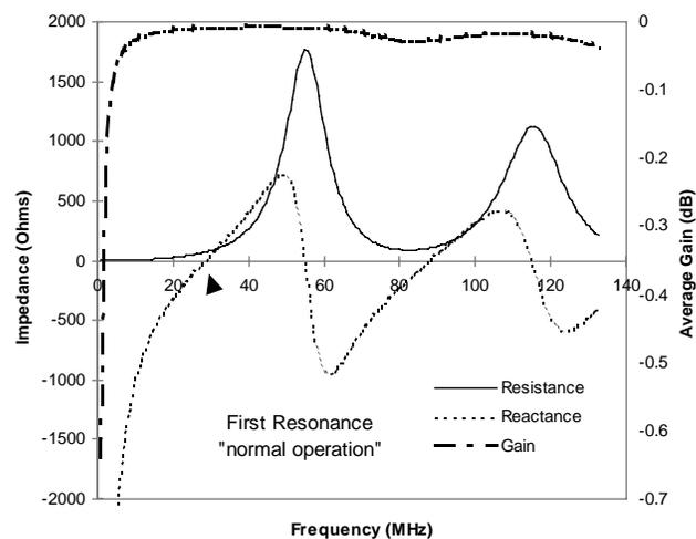
Figure 6 Gain and impedance spectrum of a standard dipole antenna.
