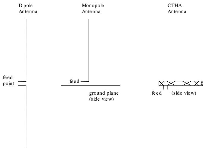
Figure 2 Height comparison illustration of the CTHA and conventional antennas.
