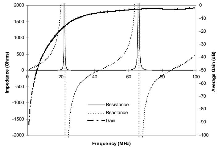
Figure 7 Gain and impedance spectrum for a CTHA.
