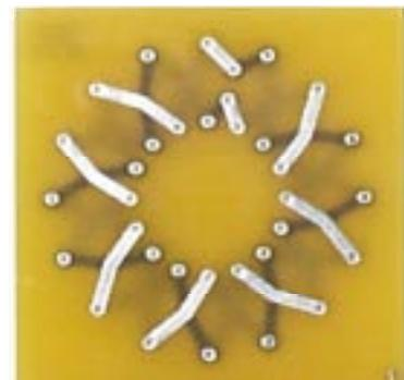
Figure 4 Multilayer printed circuit board version (<1 in<sup>2</sup>) of the CTHA for wireless computer LAN.
