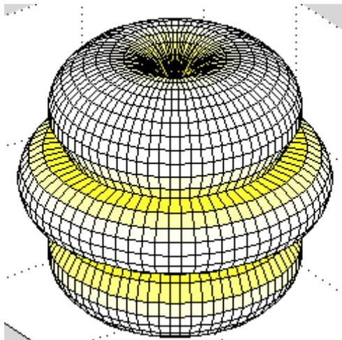
Figure 10 Third resonance far field pattern of theta-oriented gain for a dipole antenna.
