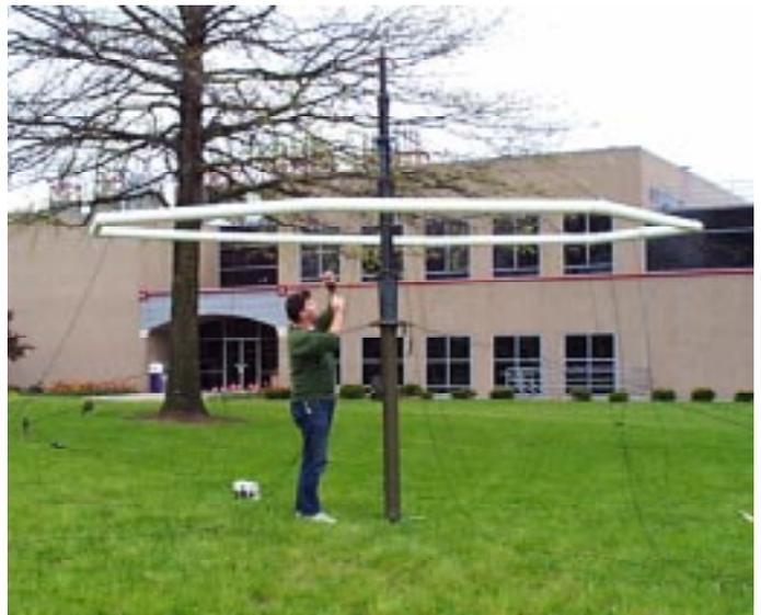
Figure 3 A 500 kHz CTHA deployed by one person which would replace a 300 m dipole.
